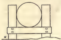
FIG. 36.—Sewerage pipe on trestle foundation.
